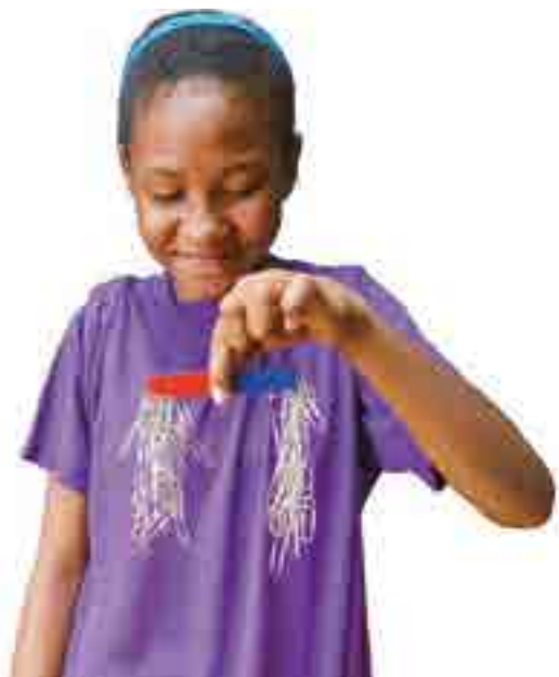
The poles attract clips much more than the other parts of the magnet.
