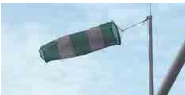
A windsock is used to tell wind direction and speed.
