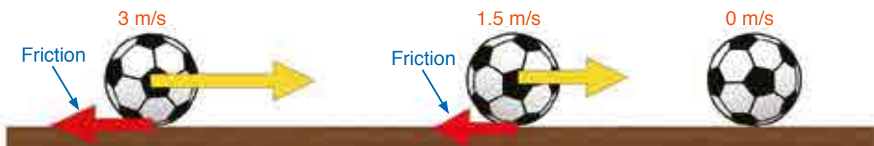
A friction makes a moving ball slow down.
