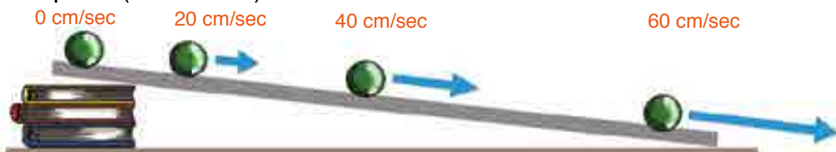
A marble increases speed as it rolls down the ramp.
